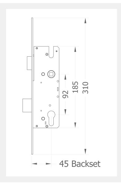
Backsets on multipoint door locks are determined by the distance from the faceplate to the centre line of the spindle or Euro cylinder, then plus 18mm for the overall depth of the lock case. This is shown on the drawing on the right - 45mm being the backset.
